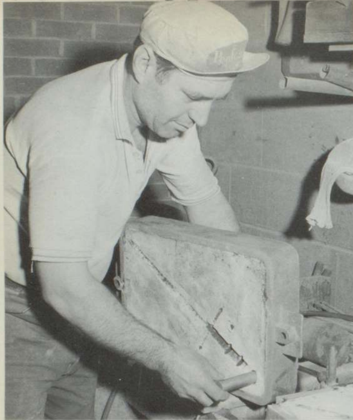
In a small Toronto foundry a mould maker prepares the sand mould for an aluminum alloy pike head, one of 11 weapons being reproduced in quantity for the tattoo by Mr. Denby. (CF-66-353-1)
